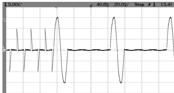
Figure 3 ZFPF Waveform Changing Modes from PF to ZF at 25% Duty Cycle
