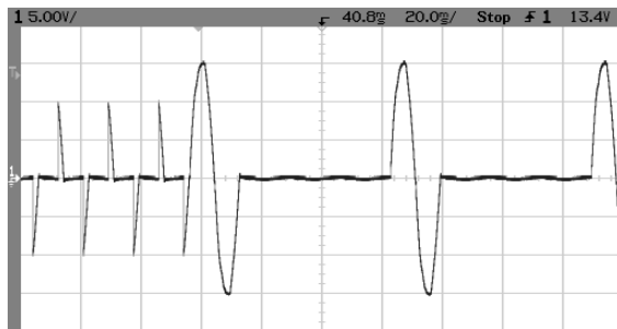
Figure 6 ZFPF Waveform Changing Modes from PF to ZF at 25% Duty Cycle
