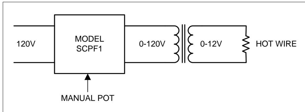
Figure 1 – Typical SCR controlled “Hot Wire” circuit
