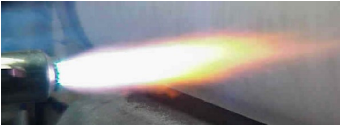
Figure 1 - Example of Plasma Spraying (Photo courtesy of White Engineering Surfaces Corp.)
